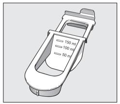
An insert is supplied in the drum of the washer.
